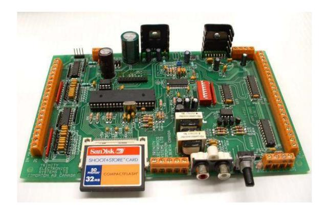
The MP3-445 is a highly versatile, highly configurable MP3 player and automation interface with an onboard audio amplifier, and extensive electrical input and output options. It can be everything from a doorbell, to the control center for a complex public multimedia display. It can operate independently, or you can use the built in serial interface to have it control other devices, or be controlled by other devices, including computers.
