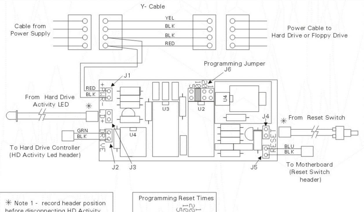
\*\* Note 1 - record header position before disconnecting HD Activity Led and Reset Switch connectors from HD controller and motherboard
